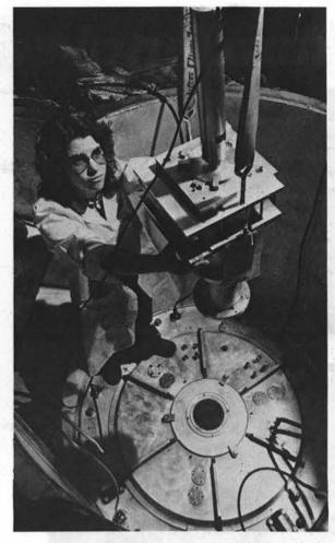
GINA NOACK (5244 - ESA) guides pin-hole camera into position for laser alignment on diode assembly of Proto I.
